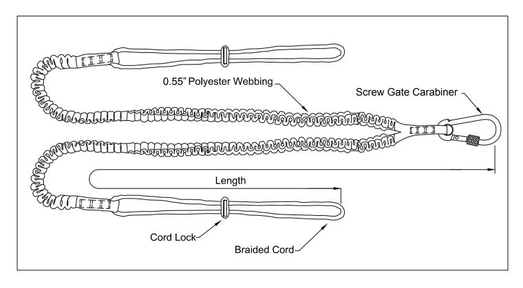
Convenient stretch lanyard for tool holding
