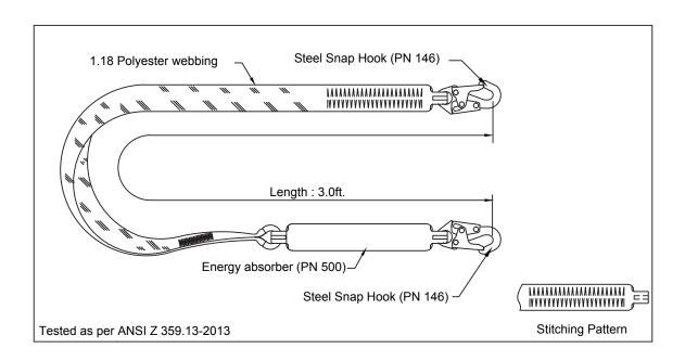
Single leg lanyard incorporated with shock absorber.
