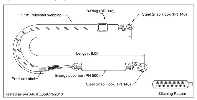
Single leg lanyard incorporated with shock absorber.
