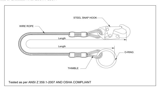
Made of PVC coated Galvanized steel
