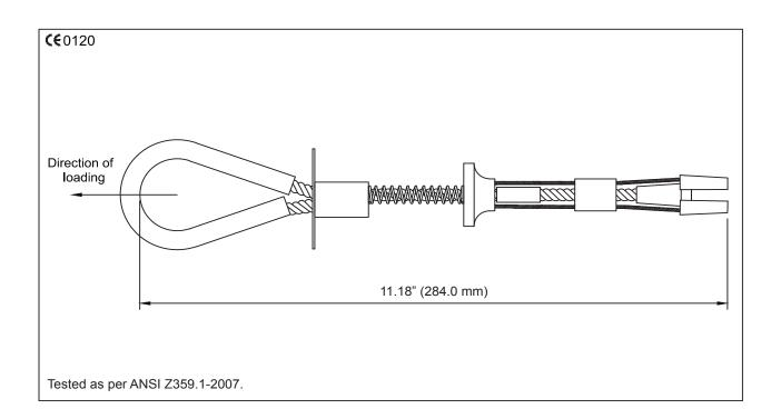
Anchor is capable of being installed on concrete having minimum thickness of 5.9"
