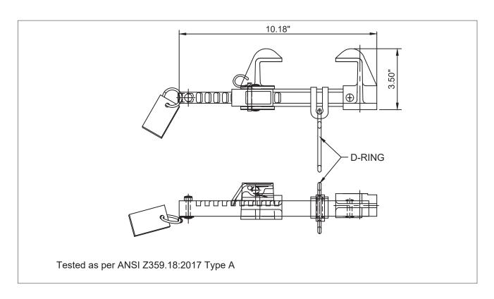
Anchor capable of being installed on flange of beams.
