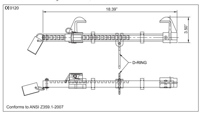
Anchor capable of being installed on flange of beams. Adjustment of the jaw to DESIGN:
