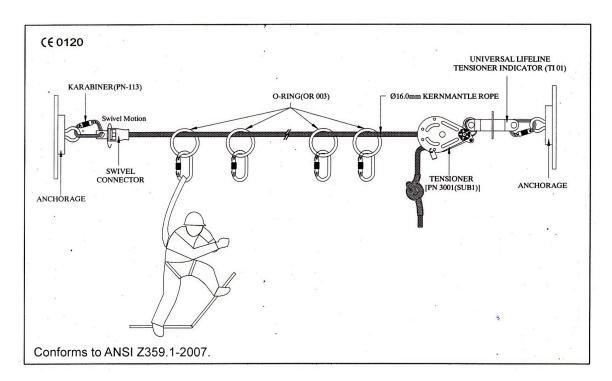
Temporary horizontal lifeline consisting of 0.63" diameter Kernmantle rope having a swivel brass connector at one end of the lifeline and a specially designed tensioner at the other end.
