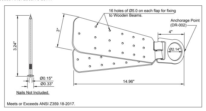
An ideal anchorage device to be fixed on wooden beams used in roofing.
