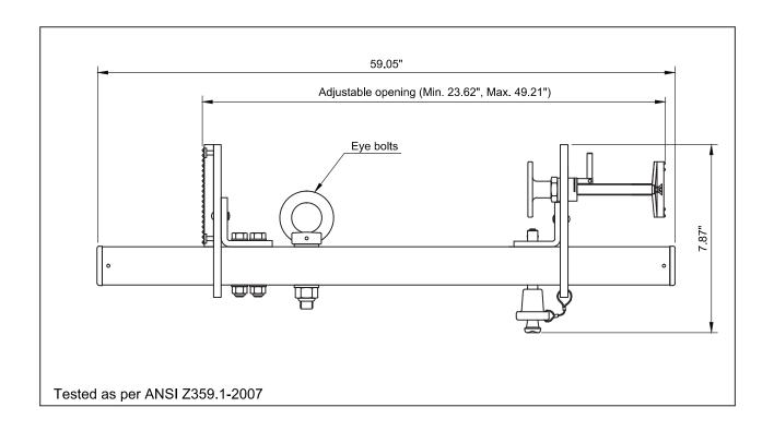
Door/window anchor is compressed against the door or window frame
