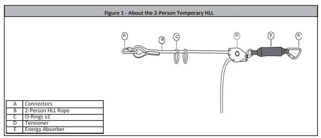
When properly tensioned, the lifeline will react to a fall event of up to two workers by combining the energy absorbing properties of the lifeline energy absorber, the lifeline, and the worker's personal energy absorber. During a fall event, the stretch of the lifeline and the expansion of the user's PFAS will result in reduced forces to the anchor and to the user's body.
