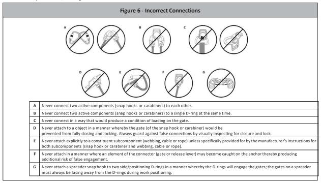
Connectors: Only use self-locking snap hooks, rebar hooks, and carabiners with this equipment. Only use connectors that are suitable to each application. Ensure all connections are compatible in size, shape and strength. Do not use equipment that is not compatible. Visually ensure all connectors close and lock completely. Connectors (snap hooks, rebar hooks, and carabiners) are designed for use only as specified in this manual.
