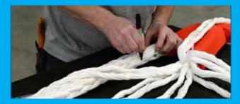
2. From the entry point, skip one strand down the rope and mark two strands with the same twist direction.
