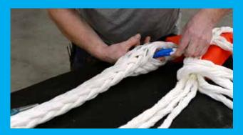
The three pairs of strands closest to the inside of the eye will be routed first through the entry point.
