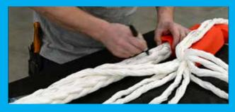
1. Mark the centerline and the entry point for the splice. The entry point should be on the side of the standing leg facing the free end of the rope that forms the eye. The entry point is defined by counting two strands on the right hand side of the centerline: one z-strand and one s-strand. Mark the point after s-strand.
