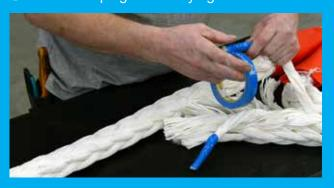
1. Tape up each of the strand ends of the free end of the rope.
