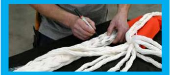
Repeat this step in a zigzag movement following the circumference of the rope. 3 times 2 s-strands (and 3 times 2 z-strands will be marked. These marks will be used as exit points.
