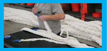
2. Then these three pairs of strands are uncoupled into six individual strands. Drop one strand in each pair and tuck the remaining three individual strands twice more.
